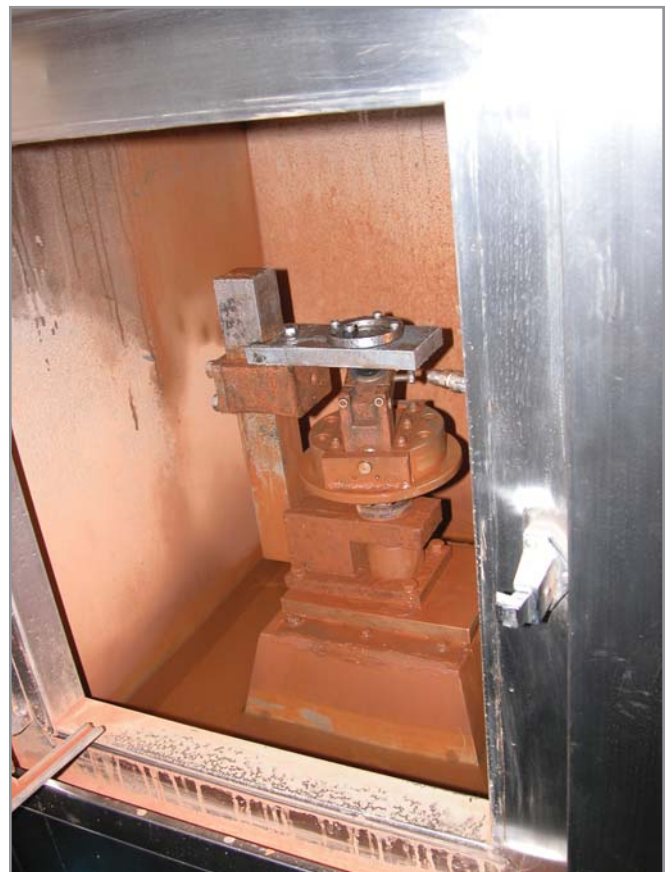
Chassis parts are tested for wear with a special mud-spray tester and a salt-spray tester.
