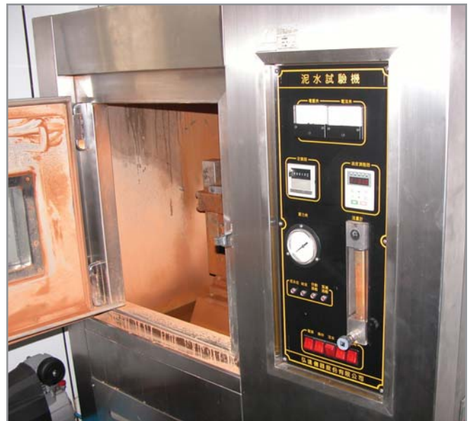
Chassis parts are tested for wear with a special mud-spray tester and a salt-spray tester.
